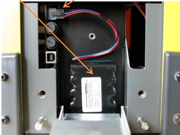
The battery can now be removed and replaced. Refit in reverse order. Please check your local regulation for disposal of the battery.
