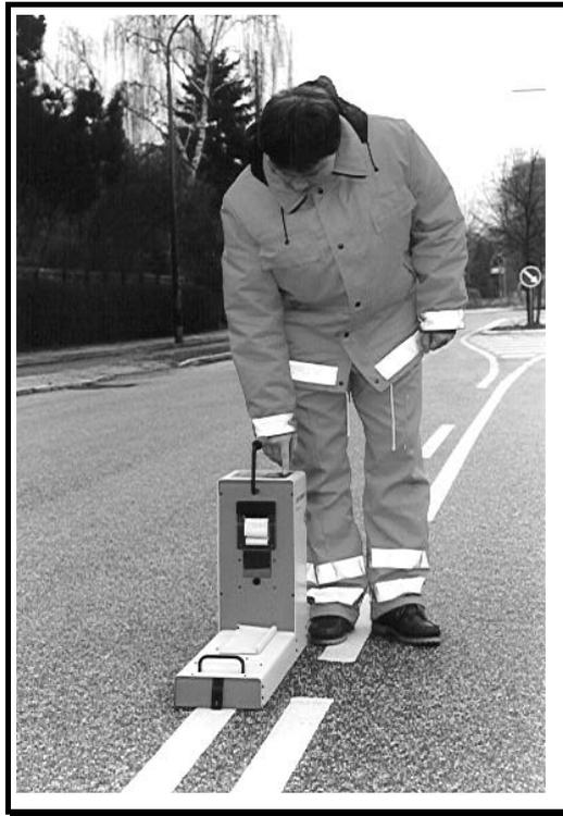
The operation of the Retrometer is very simple and requires a minimum of instruction. An error message or warning is given in case of unreliable or erroneous measurement.
