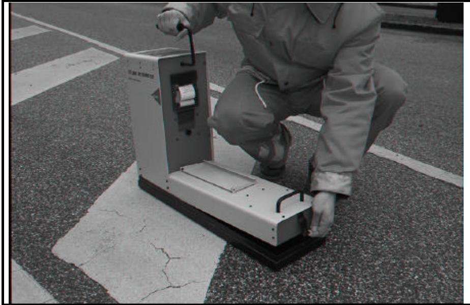
Always store the reference calibration unit in a dry and clean environment. At regular intervals the traceable calibration value must be transferred from the reference calibration unit to the control calibration unit.
