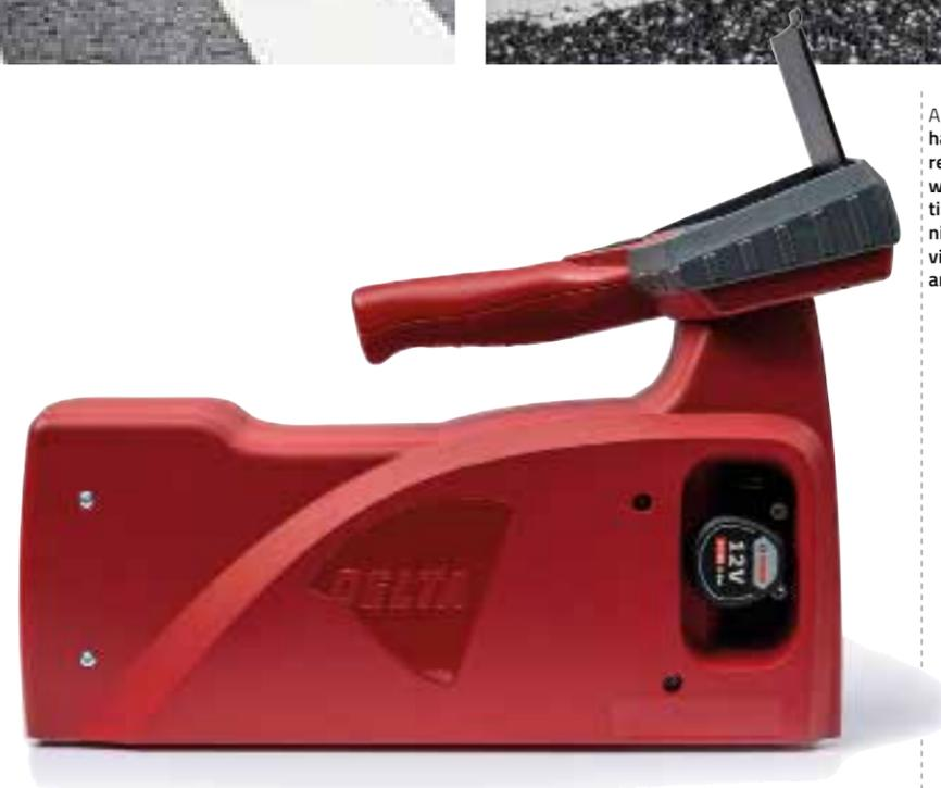
Above: Delta's new handheld LTL3000 retroreflectometer will measure night-time color as well as night and daytime visibility in both dry and wet conditions
