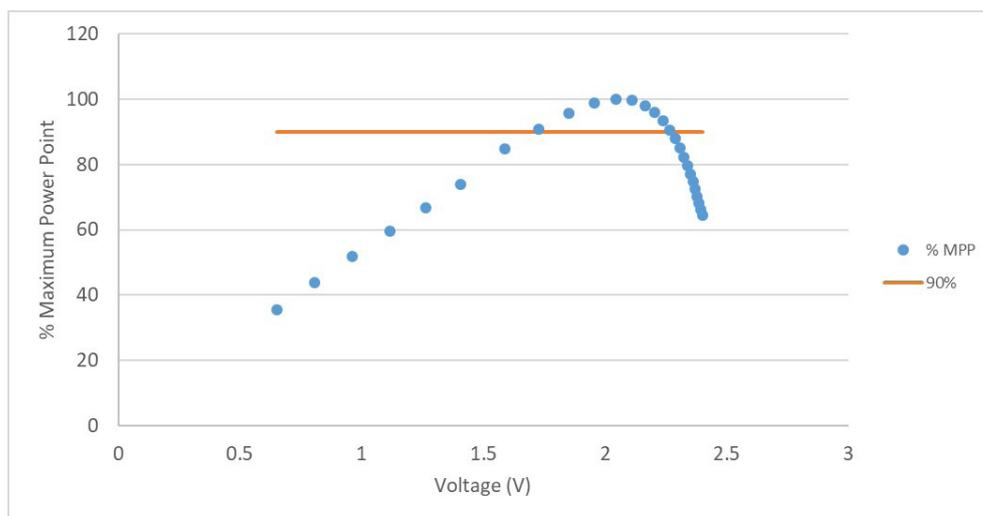
Maximum power point and the >90% efficiency operating range of a AM1417 solar cell.
