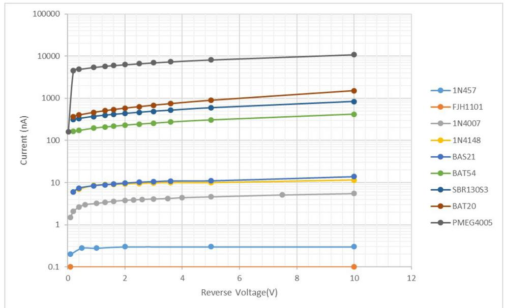
The current through the diode as a function of the applied reverse voltage.
