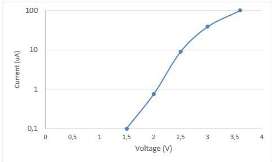
The current consumption of a solar cell in dark as a function of applied reverse voltage.
