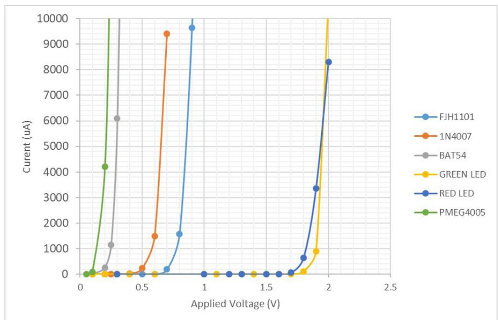
Forward Voltage drop of different types of diodes.
