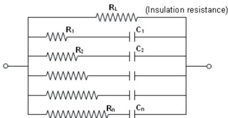
Electrical model of a supercapacitor.
