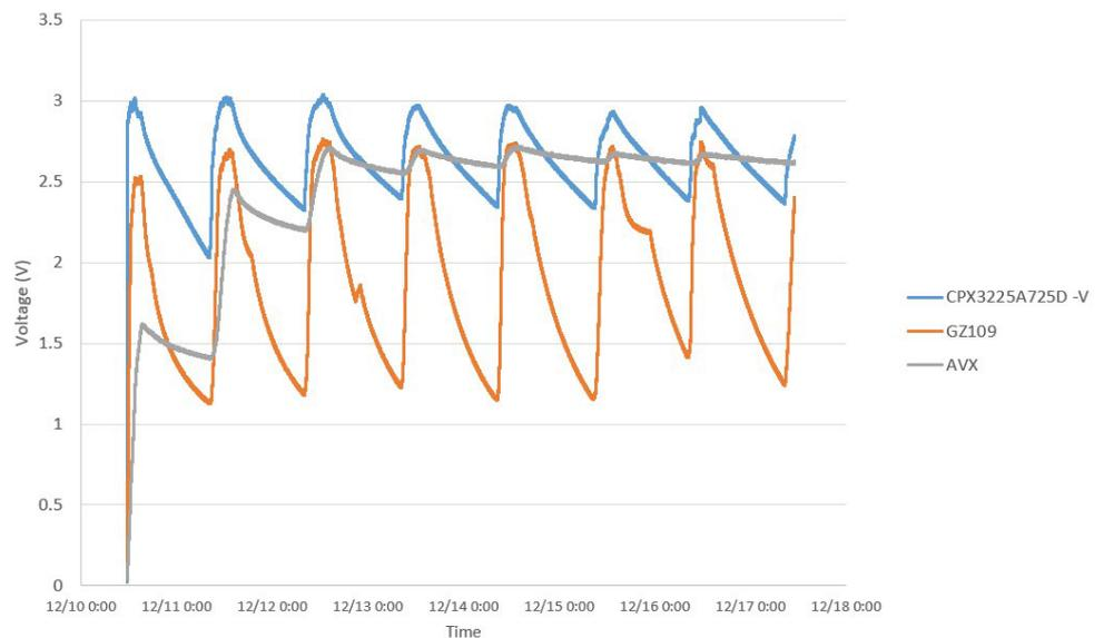
Charing of 7.5mF, 120mF and 2F units using direct coupling to solar cells.
