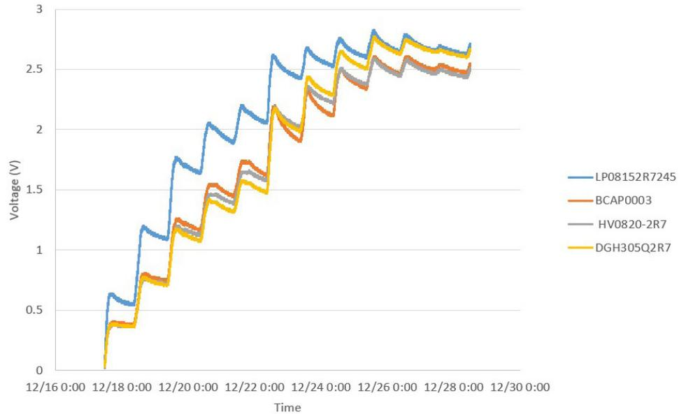
The charging of 3F capacitors using direct coupling to solar cells.
